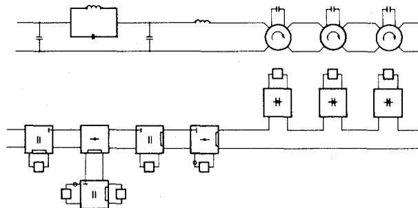
Fig. 5. Realization of a WD low-pass-all-pass branch.
