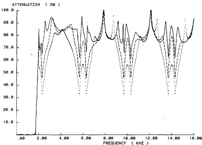
Fig. 2. Response of four-channel transmultiplexer filter designed by the Bellanger method. The coefficients of the filter in one channel are truncated to: — = 16 bits, - - - = 12 bits, ··· = 10 bits.
