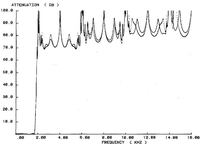
Fig. 3. Response of four-channel transmultiplexer filter with WD all-pass-low-pass sections. The coefficients of the filter in one channel are truncated to: — = 16 and 12 bits, ··· = 10 bits.
