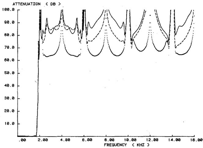
Fig. 6. Response of 60-channel transmultiplexer filter with four WD all-pass sections. All coefficients are truncated to: — = 12 bits, --- = 10 bits, ... = 8 bits.
