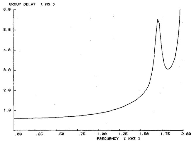
Fig. 7. Group delay of 60-channel transmultiplexer filter.
